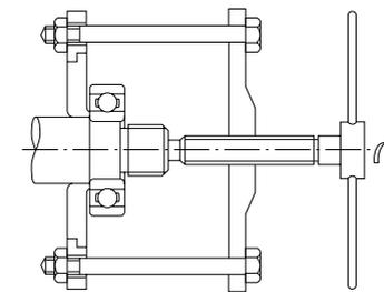
**Fig. 14.13 Removal of Inner Ring Using Withdrawal Tool (1)**
