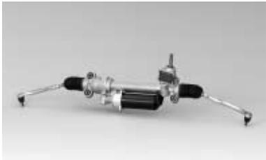
Offset Ball Screw Type Electric Power Steering
