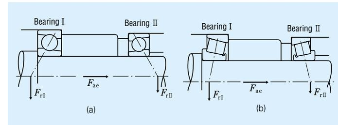
Fig. 5.12 Loads in Opposed Duplex Arrangement
