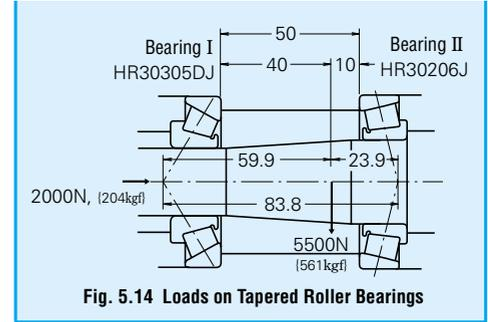
Fig. 5.14 Loads on Tapered Roller Bearings
