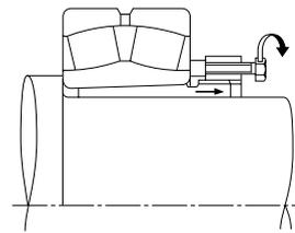
Fig. 14.17 Removal of Withdrawal Sleeve Using Withdrawal Nut (2)
