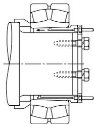
Fig. 14.7 Mounting with Special Sleeve and Hydraulic Pressure
