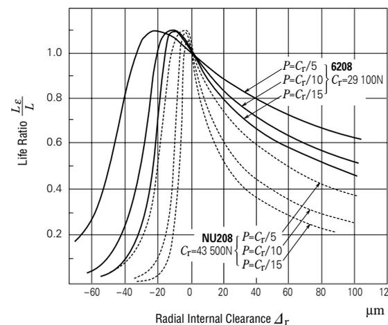
Fig. 15.13 Radial Internal Clearance and Life Ratio
