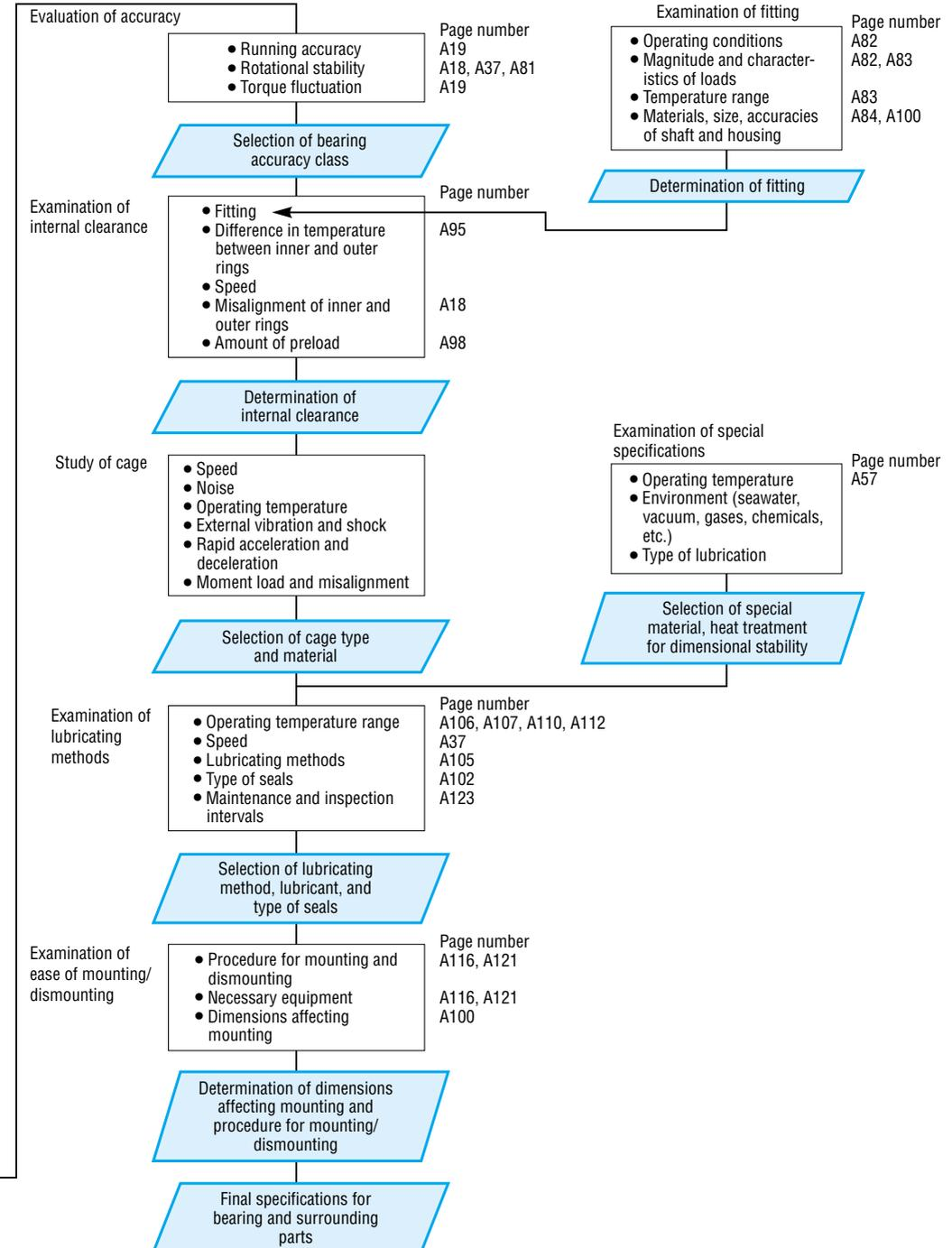
Fig. 2.1 Flow Chart for Selection of Rolling Bearings
