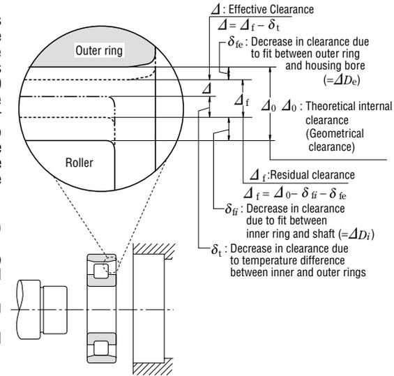
**Fig. 9.2 Changes in Radial Internal Clearance of Bearings**
