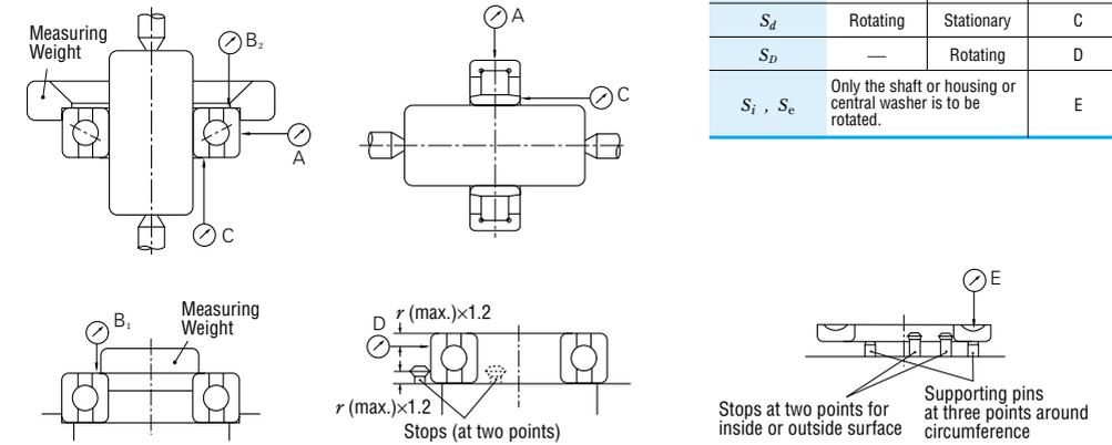
Fig. 8.1 Measuring Methods for Running Accuracy (summarized)
