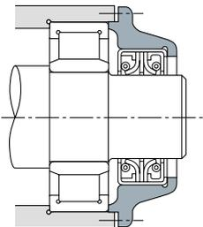
Fig. 11.9 Example of Application of Oil Seal (2)
