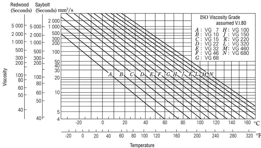
Fig. 12.11 Temperature-Viscosity Chart
