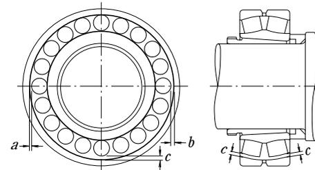
Fig. 14.9 Measuring Clearance in Large Spherical Roller Bearing
