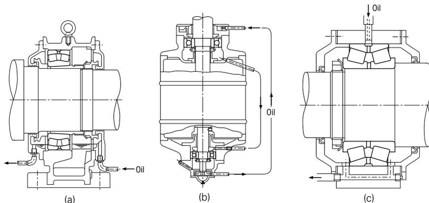
Fig. 12.7 Circulating Lubrication
