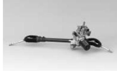
Pinion Type Electric Power Steering
