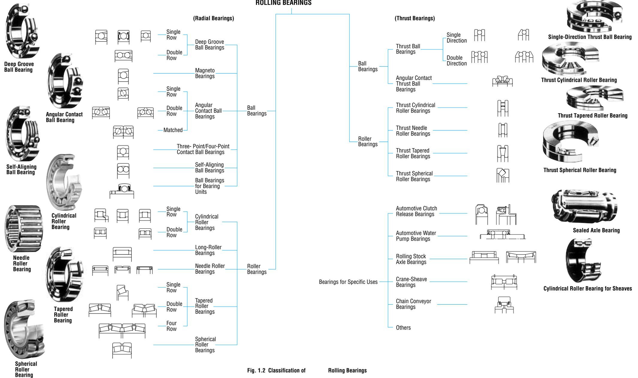
Fig. 1.2 Classification of Rolling Bearings
