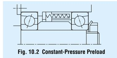
Fig. 10.2 Constant-Pressure Preload
