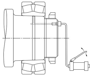
Fig. 14.19 Removal Using Oil Injection Hydraulic Pump
