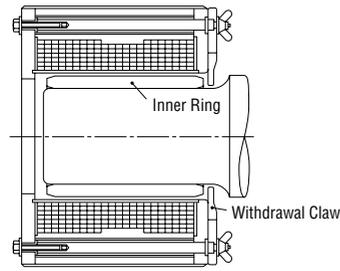
Fig. 14.15 Removal of Inner Ring Using Induction Heater
