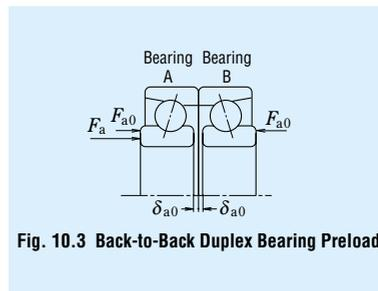
Fig. 10.3 Back-to-Back Duplex Bearing Preload
