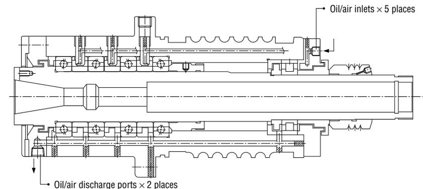
Fig. 12.10 Oil/Air Lubrication
