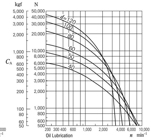
Fig. 5.13 Permissible Axial Load for Cylindrical Roller Bearings
