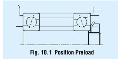
Fig. 10.1 Position Preload
