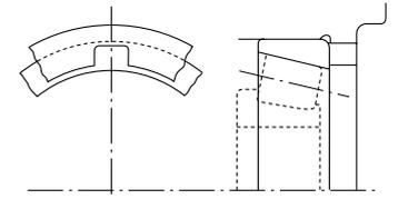
**Fig. 14.11 Removal Notches**
