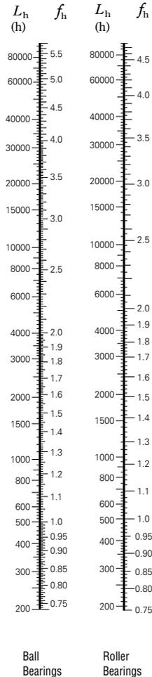
Fig. 5.4 Fatigue Life Factor and Fatigue Life
