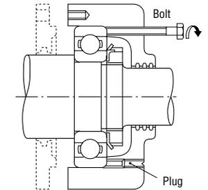
**Fig. 14.10 Removal of Outer Ring with Dismounting Bolts**
