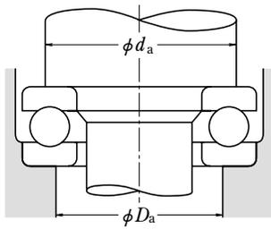
Fig. 11.3 Face Supporting Diameters for Thrust Ball Bearings
