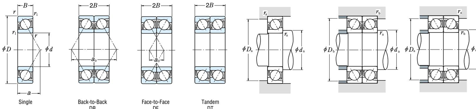
Dynamic Equivalent Load P = XF<sub>r</sub> + YF<sub>a</sub>
