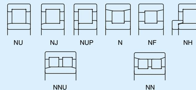
Types NU, N, NNU, and NN are suitable as free-end bearings. Types NJ and NF can sustain limited axial loads in one direction. Types NH and NUP can be used as fixed-end bearings.
