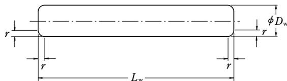
**Remarks** The figure shows an example of a flat-end long cylindrical roller.
