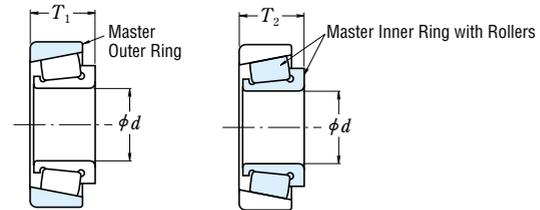
**Table 8. 4 Tolerances for Inch Design Tapered Roller Bearings**
