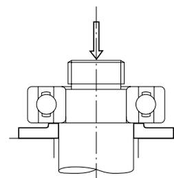
**Fig. 14.12 Removal of Inner Ring Using a Press**
