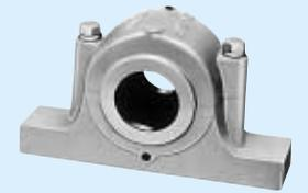
These have the same dimensions as those of types SN5 and SN6. To increase the bearing box strength, no material is removed from the top or bottom of the base, so mounting holes can be drilled anywhere.
