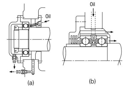
Fig. 12.8 Jet Lubrication
