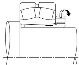
Fig. 14.16 Removal of Withdrawal Sleeve Using Withdrawal Nut (1)
