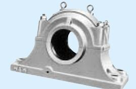
These are large and made for heavy loads. The standard ones have double seals and four mounting bolt holes. For types SD2C and SD3C, the bore diameters on the two sides are different.
