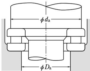
Fig. 11.4 Face Supporting Diameters for Thrust Roller Bearings
