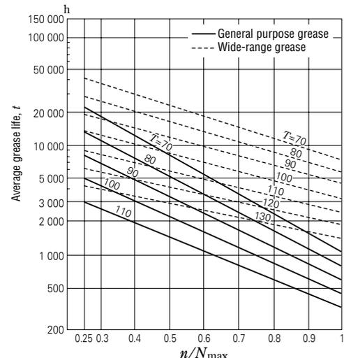
**Fig. 12.3** Grease Life of Sealed Ball Bearings
