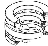
There are also thrust ball bearings with an aligning seat washer beneath the housing washer in order to compensate for shaft misalignment or mounting error. Pressed steel cages are usually used in the smaller bearings and machined cages in the larger
