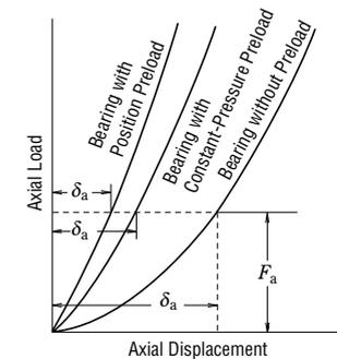
Fig. 10.6 Comparison of Rigidities and Preloading Methods
