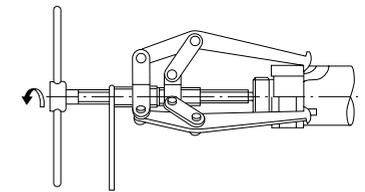
**Fig. 14.14 Removal of Inner Ring Using Withdrawal Tool (2)**
