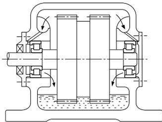
Fig. 12.6 Splash Lubrication
