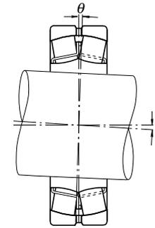
Fig. 3.4 Permissible Misalignment of Spherical Roller Bearings
