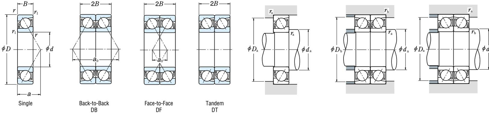
Dynamic Equivalent Load P = X\*F\_r + Y\*F\_a. Table with columns for Contact Angle, i\*F\_a/C\_o\*r, e, Single/DT, and DB/DF load factors X and Y for various contact angles (15, 25, 30, 40 degrees).
