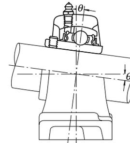
Fig. 3.5 Permissible Misalignment of Ball Bearing Units
