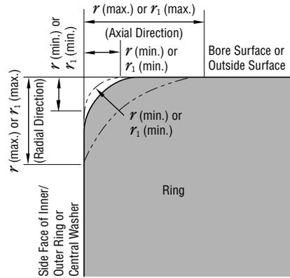
$r$  : Chamfer Dimension of Inner/Outer Ring
