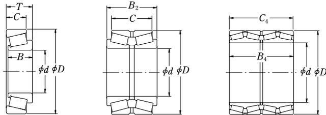
**Tapered Roller Bearings and Combined Bearing Width**
