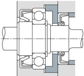
Fig. 11.8 Example of Application of Oil Seal (1)
