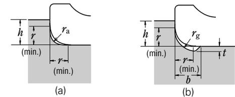
**Fig. 11.2 Chamfer Dimensions, Fillet Radius, and Shoulder Height**
