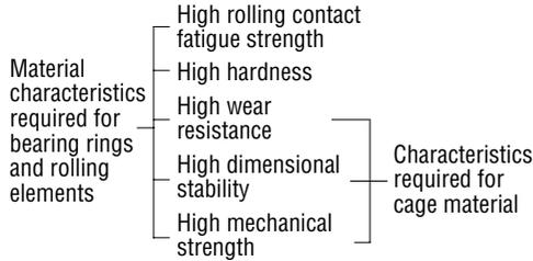
Other necessary characteristics, such as easy production, shock and heat resistance, and corrosion resistance, are required depending on individual applications.
