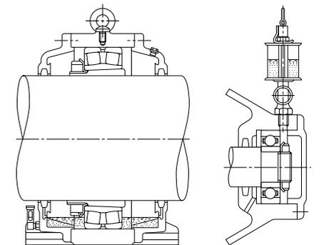
**Fig. 12.4** Oil Bath Lubrication
