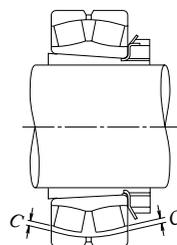
Fig. 14.8 Clearance Measurement of Spherical Roller Bearing
