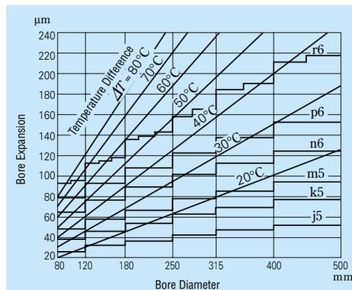
Fig. 14.3 Temperature and Thermal Expansion of Inner Ring
