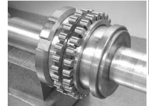
Fig. 1.13 Setting of GN Gauge
