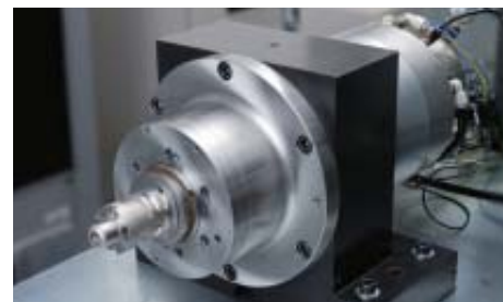
NSK Spindle that achieved 4 million d_m n using ceramic ball bearings
