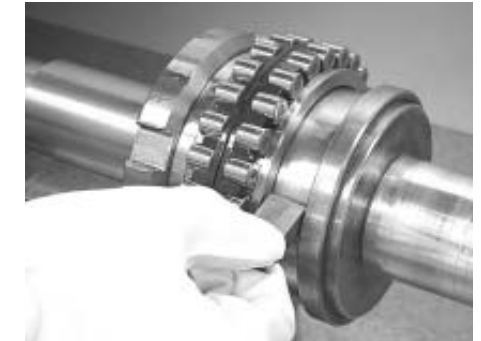
Fig. 1.15 Measurement of Spacer Width
