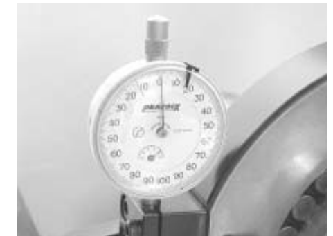
Fig. 1.15 Measurement of Spacer Width
