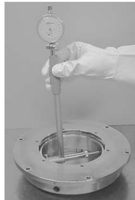
Fig. 1.10 Zero Setting of Cylinder Gauge
