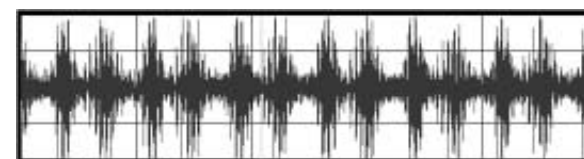
Sound waveform of a scratched bearing
