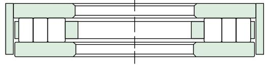
This type of bearing undergoes static loading in normal applications. Our static capacities are based on a total permanent deformation of .0002 inch per inch of roller diameter and is not the ABMA basic capacity.
