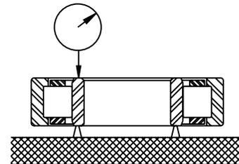
**Reference Side Runout With Bore** - Mount the bearing on an arbor having a taper of .0001 to .0002 inch in diameter per inch of length, and position the arbor between two accurate centers so that it can be rotated. Apply an indicator against the reference side of the inner race on a diameter as equal to the raceway diameter as possible. Take indicator readings while rotating the inner ring one revolution. Correction must be made for inaccuracy of the arbor.
