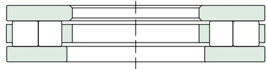
The sizes range from 1 to 22 inches I.D. and 2.125 to 34 inches O.D. with dynamic capacities from 10,000 lbs. to 1,620,000 lbs. These bearings are used in a variety of applications such as extruder gear drives, pumps, crane hook swivels and machine tools.
