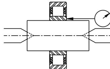
**Outside Diameter of Outer Race** - For determining outside diameter, use apparatus arranged for two-point measuring. Measure single diameters in at least three angular directions and two radial planes. In this manner  $D_{min}$  and  $D_{max}$  are established, from which the mean diameter is obtained by:
