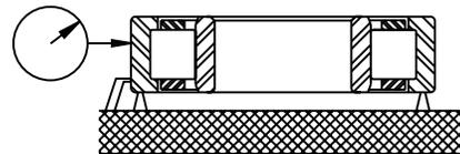
**Inner Race Radial Runout** - Mount the bearing on an arbor having a taper of .0001 to .0002 inch in diameter per inch of length and position the arbor between two accurate centers, or other suitable supports, so that it can be rotated. Place an indicator against the OD and in the plane of the centerline. Hold the outer race stationary and take indicator readings while rotating the inner race one revolution.
