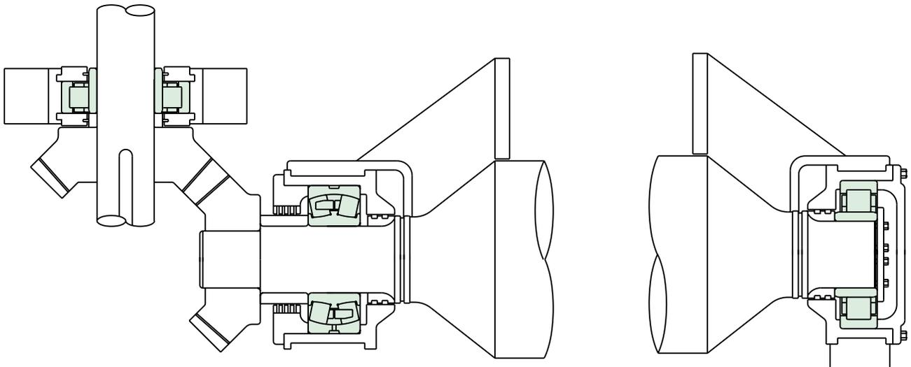
***Rolling Mill Runout Table Applications
