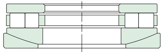
The standard “AT” type is recommended for vertical shaft applications. Where the alignment feature is required in some horizontal shaft applications, the convex aligning plate may ride on the shaft and the plate should be modified to provide a satisfactory bearing surface in the bore. This is usually achieved by the installation of a brass bushing into the bore of the plate.
