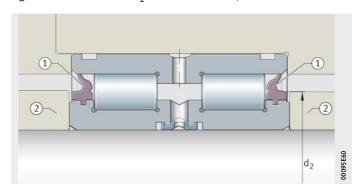
① Sealing ring ② Spacer ring (alternatively shaft shoulder)
