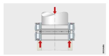
Figure 5 Application of mounting forces
