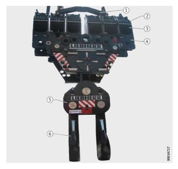
① Hook crossbeam ② Pulley set ③ Rope sheave ④ Upper part ⑤ Lower part ⑥ Hook
