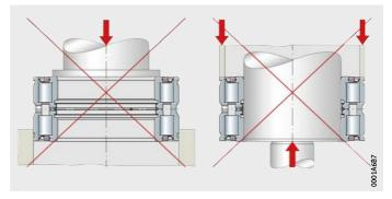
Figure 6 Impermissible mounting or dismounting methods
