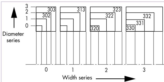
The original metric part numbering system for tapered roller bearings was based on the ISO 15 dimensional plan for radial bearings. A 5-digit part number commencing with numeral 3 describes the bearing assembly (cone and cups).
