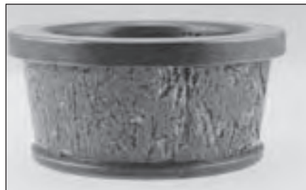
Rapid and deep spalling caused by unusually high stresses. Full race width fatigue spalling is caused by heavy loads creating a thin lubricant film and possible elevated temperatures.
