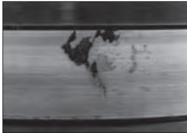
Point surface origin — Spalling from debris or raised metal exceeding the lubricant film thickness.
