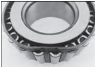
Cage deformation — Improperly installed or dropped bearing.
