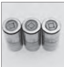
Roller end scoring — Metal-to-metal contact from breakdown of lubricant film.
