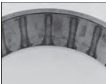
Staining — Surface stain with no significant corrosion from moisture exposure.
