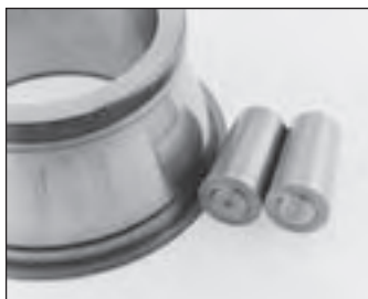
Abrasive wear — Fine abrasive particle contamination.
