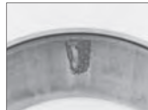
Localized spalling on the cup race from stress riser created by split housing pinch point.
