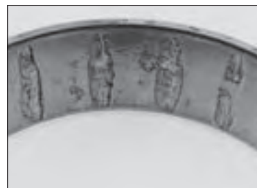
Line spalling — Roller-spaced spalling from bearings operating after etching damage.
