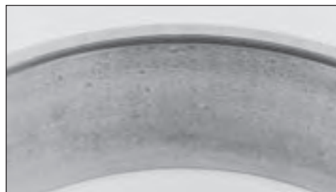
Bruising — Debris from other fatigued parts, inadequate sealing or poor maintenance.
