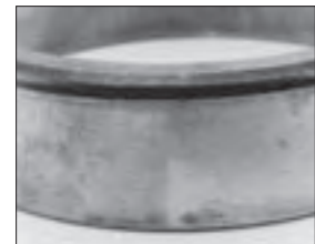
Localized spalling on the cup race from stress riser created by split housing pinch point.
