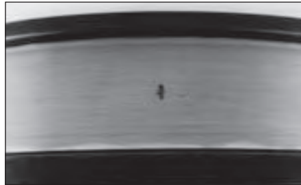
Inclusion origin — Spalling from oxides or other hard inclusions in bearing steel.
