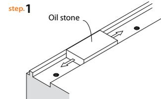
Prior to installation, the burrs, dirt, and rust preventive oil should be removed thoroughly.
