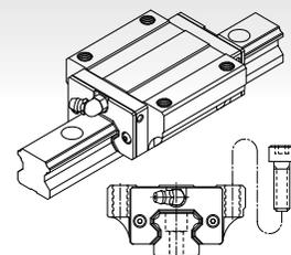
Installed from top side of carriage with the thread length longer than MSA-E type.
