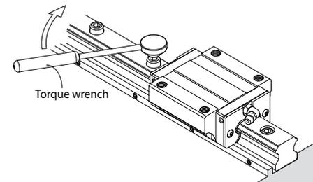
Tighten all bolts to the specified torque. The tightening sequence should start from the center to both ends. By doing this, the original accuracy could be achieved.
