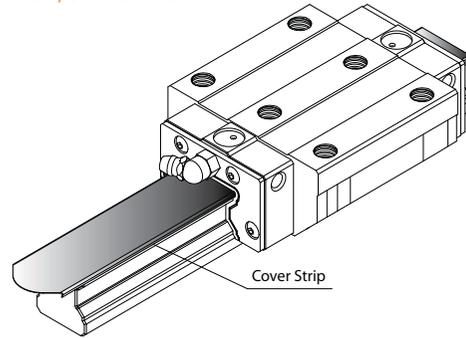
The cover strip of MSR and SMR series will increase the assembly height of rail. The increment refer to the table below.
