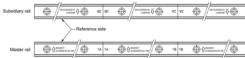
Identification of butt-joint rail
