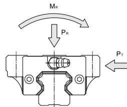
When a linear guideway system receives varying loads, the service life could be calculated in consideration of varying loads of the host-system operation conditions. The mean load ( $P_m$ ) is the load that the service life is equivalent to the system which under the varying load conditions. The equation of mean load is:
