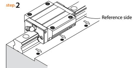
Gently place the linear guideway on the bed, and pushing it against the reference side of bed.
