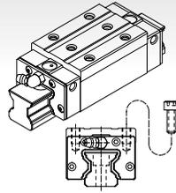
Square type with smaller width and can be installed from top side of carriage.
