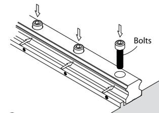
Check for correct bolt play and temporarily tighten all bolts.
