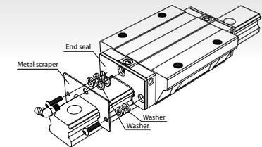
Removing spatters, iron chips, and large foreign matters as well as protecting the end seals.
