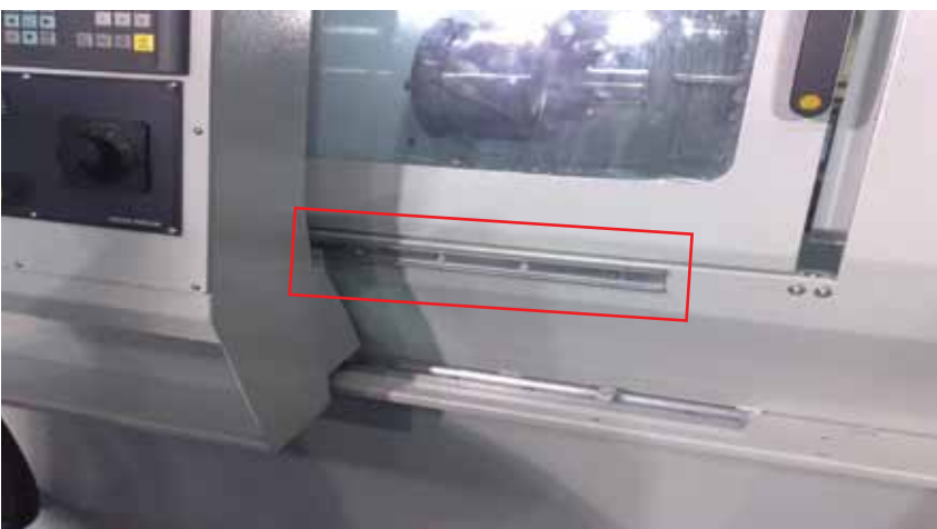
HEAVY DUTY RAIL RB 28 USED IN CNC MACHINE FOR CONSOLE MOVEMENT
