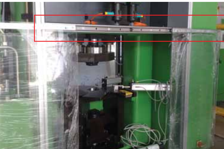
SS LINEAR SILDE RAIL USED IN MACHINE DOOR
