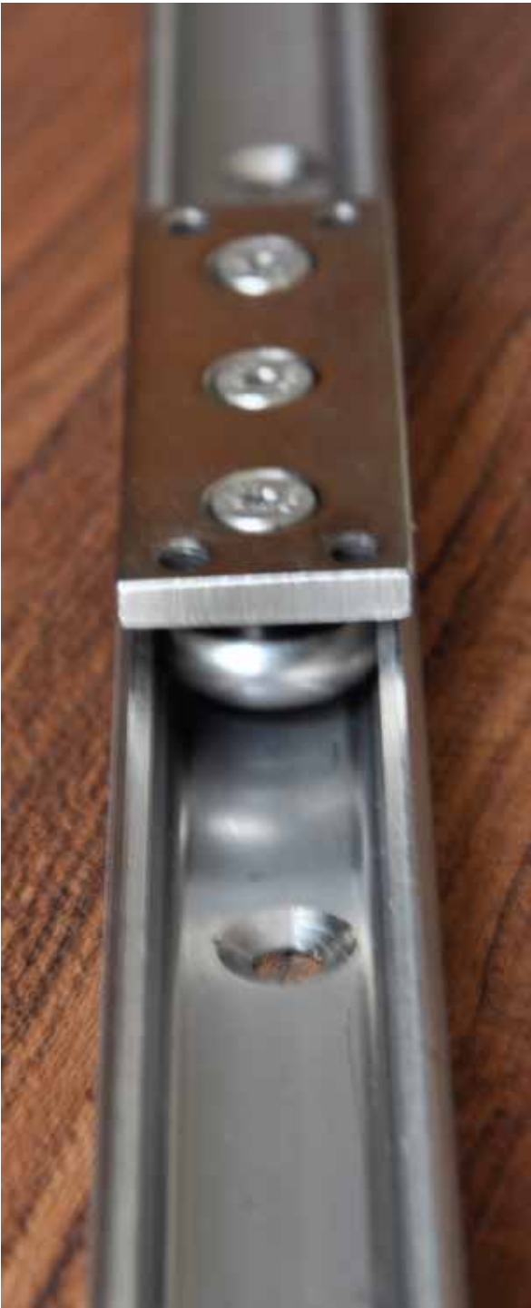
SS LINEAR SILDE RAIL USED IN MACHINE DOOR
