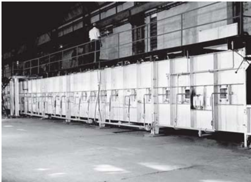
Le Four furnace for high quality patenting/galvanising
